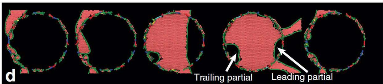
Figure 1: Cutting sequence of a spherical Ag precipitate in fcc-Cu by an edge dislocation that has dissociated in two partial dislocations. Shown in red are atoms in an hcp-configuration, i.e. stacking faults. Dislocation line segments are colored according to their type determined by DXA in OVITO, where blue segments represent full dislocations, green partials, yellow Hirth-locks, grey Lomer-Cottrell segments and red unnamed dislocation types.
